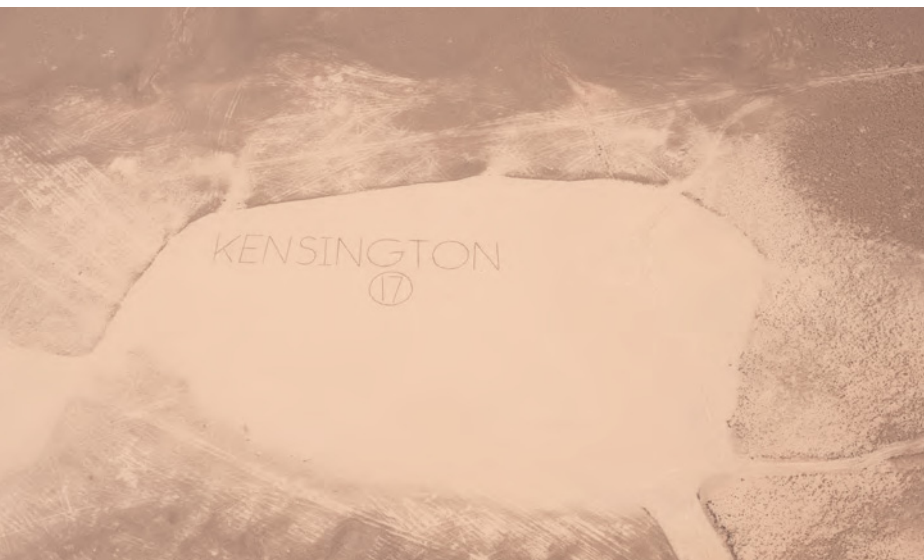
Figure 10. A landing ground for the aircraft using the Cairo–Baghdad Air Mail Route—this one called “KENSINGTON” 17—the mudpans were clear of stones and good for landing and essential for aircraft refuelling en route, as well as repair stations for replacing engines, repairing propellers and tires. Photograph: Robert Bewley, APAAME_20141015_RHB-0441, courtesy of APAAME.
